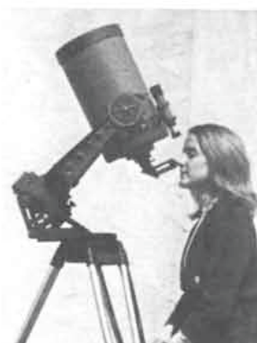
The Celestron 8, with equatorial wedge and tripod, a portable observatory for the serious amateur astronomer.
