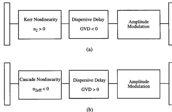
Fig. 1. Block diagrams of femtosecond KLM lasers: (a) traditional approach, (b) approach described here.
