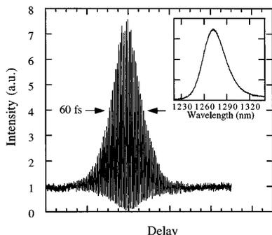
Fig. 5. Autocorrelation and power spectrum (inset) of pulses generated with prisms removed from the laser. The time-bandwidth product is  $\tau\Delta\nu = 0.4$ .
