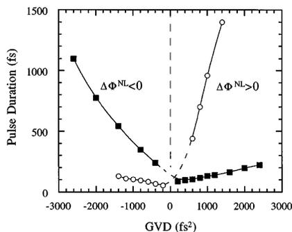
Fig. 4. Pulse duration plotted versus cavity dispersion. Open symbols, ordinary KLM; filled symbols, KLM with the cascade nonlinearity. The curves are to guide the eye, and dashed portions of the curves indicate unstable regions.
