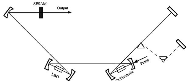
Fig. 3. Schematic of the laser: dashed lines, beam path with prisms in the cavity; solid lines, paths without prisms. SESAM, semiconductor saturable absorber mirror.
