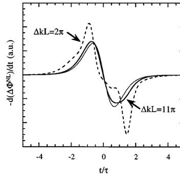
Fig. 2. Frequency sweeps generated in the cascade process with GVM equal to the pulse duration and  $\Delta kL = 2\pi$  and  $\Delta kL = 11\pi$ . The magnitude of the phase shift produced with  $\Delta kL = 2\pi$  is  $\sim 2.5$  times as large as that produced with  $\Delta kL = 11\pi$ . The fine solid curve corresponds to an instantaneous nonlinear index of refraction.
